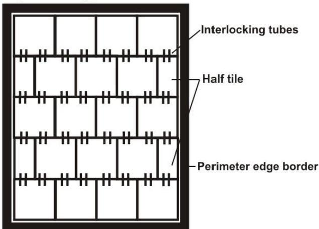
**The correct installation of Dinoflex Rubber Tiles is a staggered pattern to ensure proper alignment, a tighter fit, and reduction of vandalism.**
