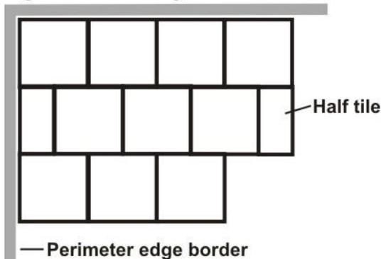
**The correct installation of Dinoflex Rubber Tiles is a staggered pattern to ensure proper alignment, a tighter fit, and reduction of vandalism.**
